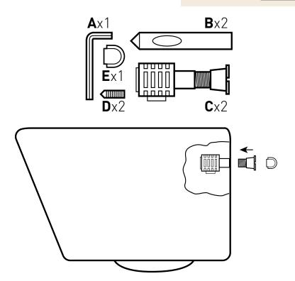
• Unscrew Part C into 2 pieces. Hold the larger part in the WC, insert the threaded part from the outside and tighten using part E. Ensure that the smaller, metal thread is pointing vertically downwards
