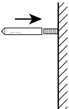
• Screw Steel Pegs, part B (x2), onto the fixing frame, ensure that the oval groove points down vertically
