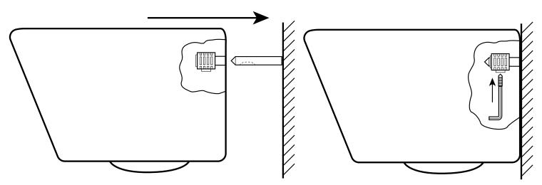
• Slide the WC onto the steel pegs
