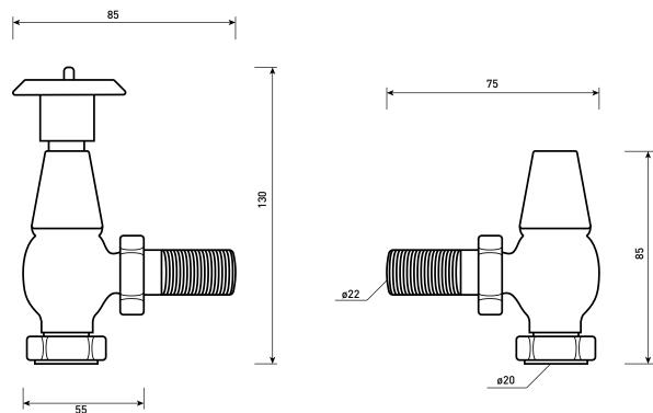
Information: The valves are not bi-directional and should be fitted to the flow side. Max working pressure: 10bar Max pressure differential: 1bar Max water temp 85°C Max ambient temp 50°C Temp adjustment 7°C - 32°C
