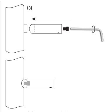
3. Insert bolts (x4) into bracket tube (x4) and screw to mounting plate on radiator using an allen key.
