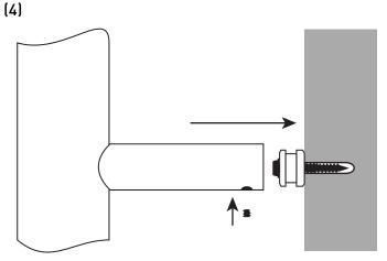
4. Offer radiator up to wall so that brackets tubes (x4) cover collars (x4). Fix together with grub screw (x4). Support radiator in place whilst performing this assembly.
