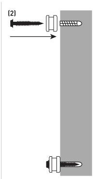
2. Insert large screw (x4) through collar (x4) and screw into wall plug (x4), ensuring a secure fitting.
