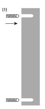
1. Measure & mark wall for mounting bracket holes (x4). Insert wall plugs (x4) into drilled holes.
