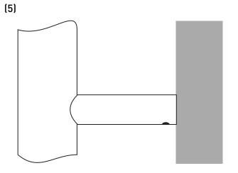
5. Ensure radiator and all parts are secure before unsupporting the radiator. Continue with plumbing of radiator.
